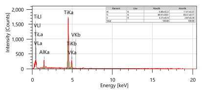
Figure 7. SEM- EDX of Ti-6Al-4V workpiece
