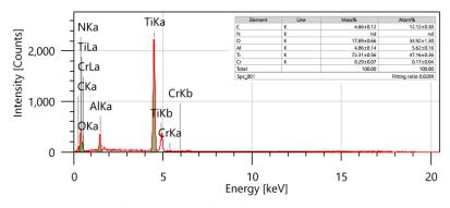
Fig. 8. SEM- EDX of machined surface after micro-EDM with WC electrode
