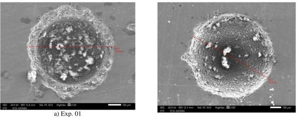
a) Exp. 01 (V=120V, C=100pF, RPM=200rpm) b) Optimal process
